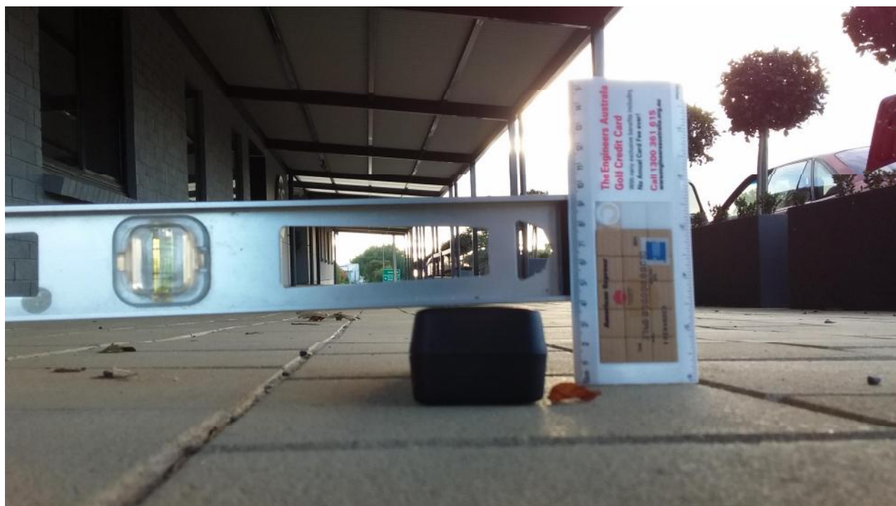
Plate 7 Crossfall 52mm in 1220mm uphill from the main door.(1:23, 4.3%)
