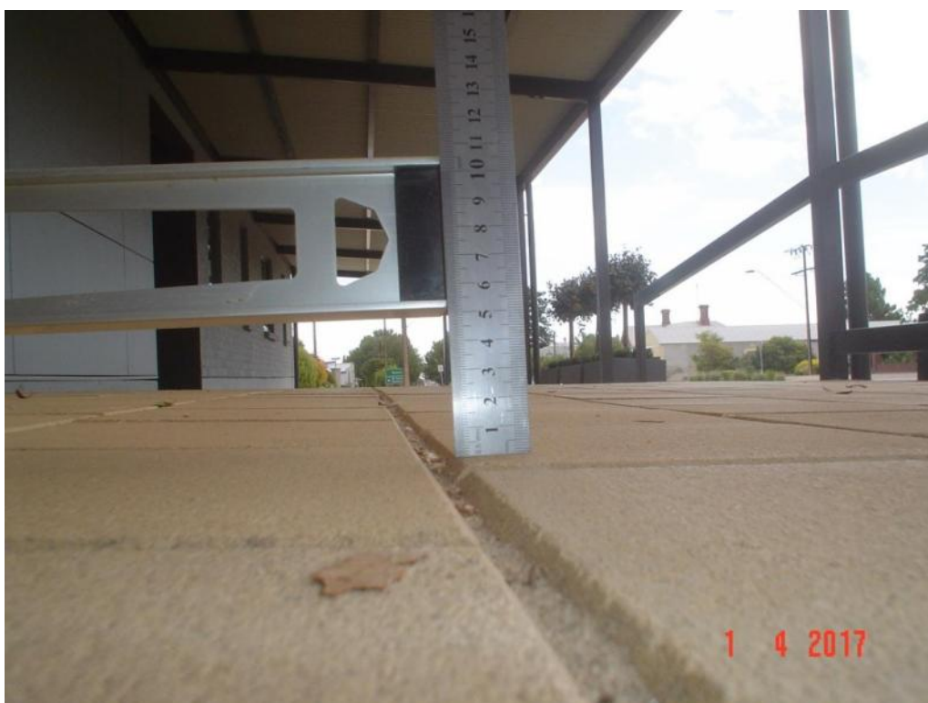
Plate 10 Crossfall at the main entrance 52mm in 1220mm. (1:23, 4.3%)
