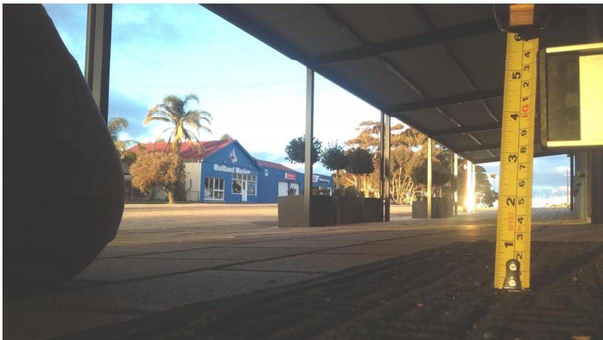
Plate 9 Crossfall 78mm in 1220mm; at the main door threshold. (1:16, 6.4%)
