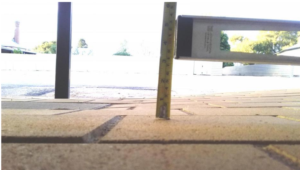
Plate 11 Longitudinal fall 78mm in 1220 downhill from the main door (1:16, 6.3%)
