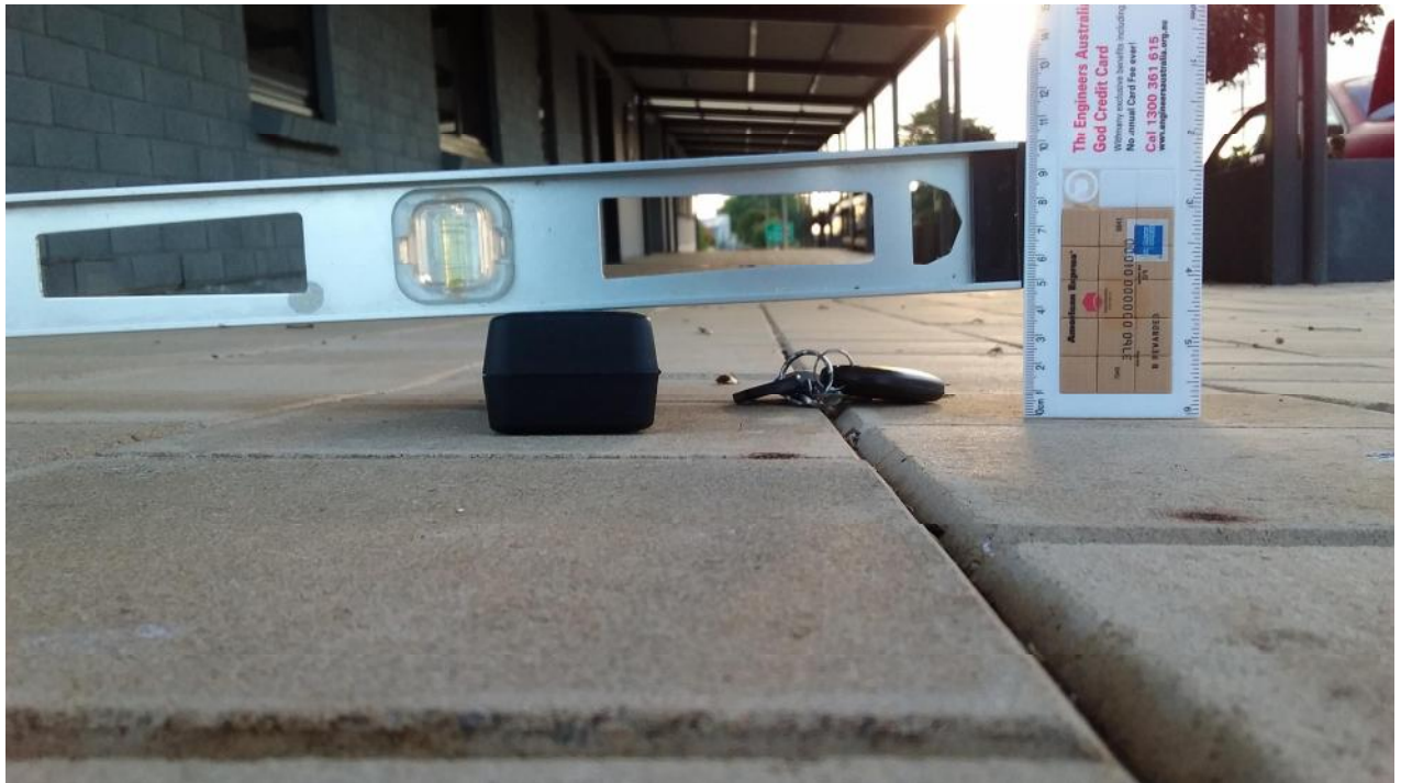
Plate 5 Crossfall downhill from the corner of building (1:16, 6.25%);
