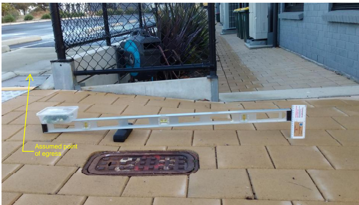
Plate 4 Longitudinal fall downhill from the disabled parking. (1:15, 6.6%)
